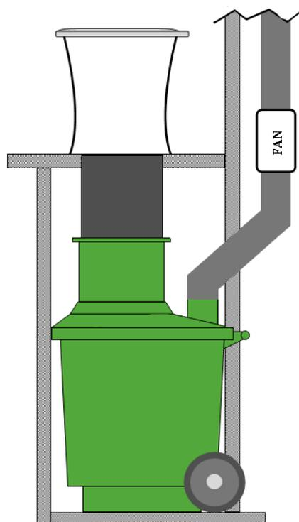
The most common way to install and service the GT System is to push the container from the back of the toilet room to its position under the seat. To locate the waste shaft, there are rails in the package to be installed to both sides of the toilet base chute hole (see picture below). These rails ensure that the shaft holds firmly in its place during use.
